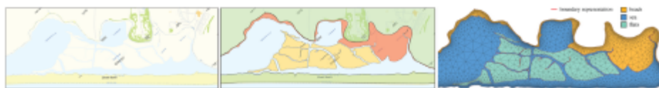
Figure 2. Left: A portion of an Ordnance Survey Street View product centred around the East Fleet region behind Chesil Beach, identified in Figure 1. Centre: The same region overlaid with vector polygon layers containing GIS generated contours of the beach and flat regions. Right: The meshed flats region accurately constrained by a metric calculated from several raster maps and polygon layers within GIS.
